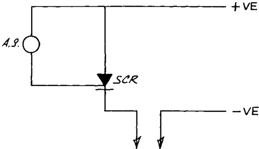
FIG. 86 ALKA SELTZER TABLET SWITCH
