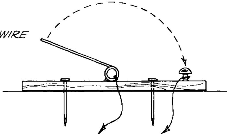
FIG. 35 MOUSETRAP RELEASE SWITCH
