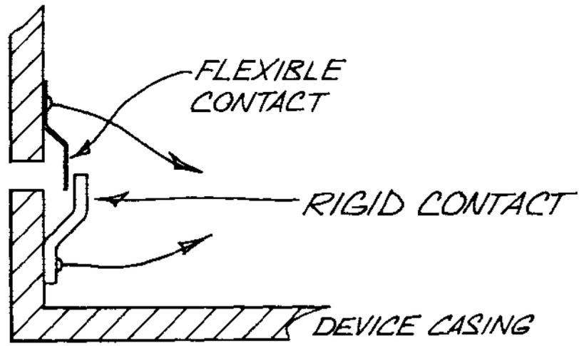
FIG. 55 ANTI-PROBE SWITCH
