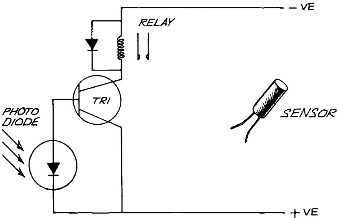
FIG. 82 INFRA-RED SENSITIVE SWITCH
