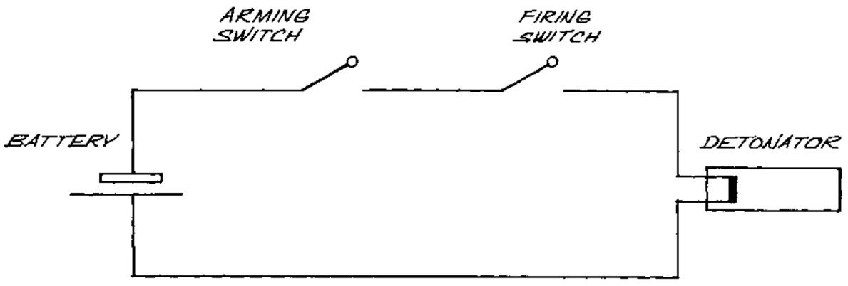
FIG. 1 BASIC I.E.D. CIRCUIT
