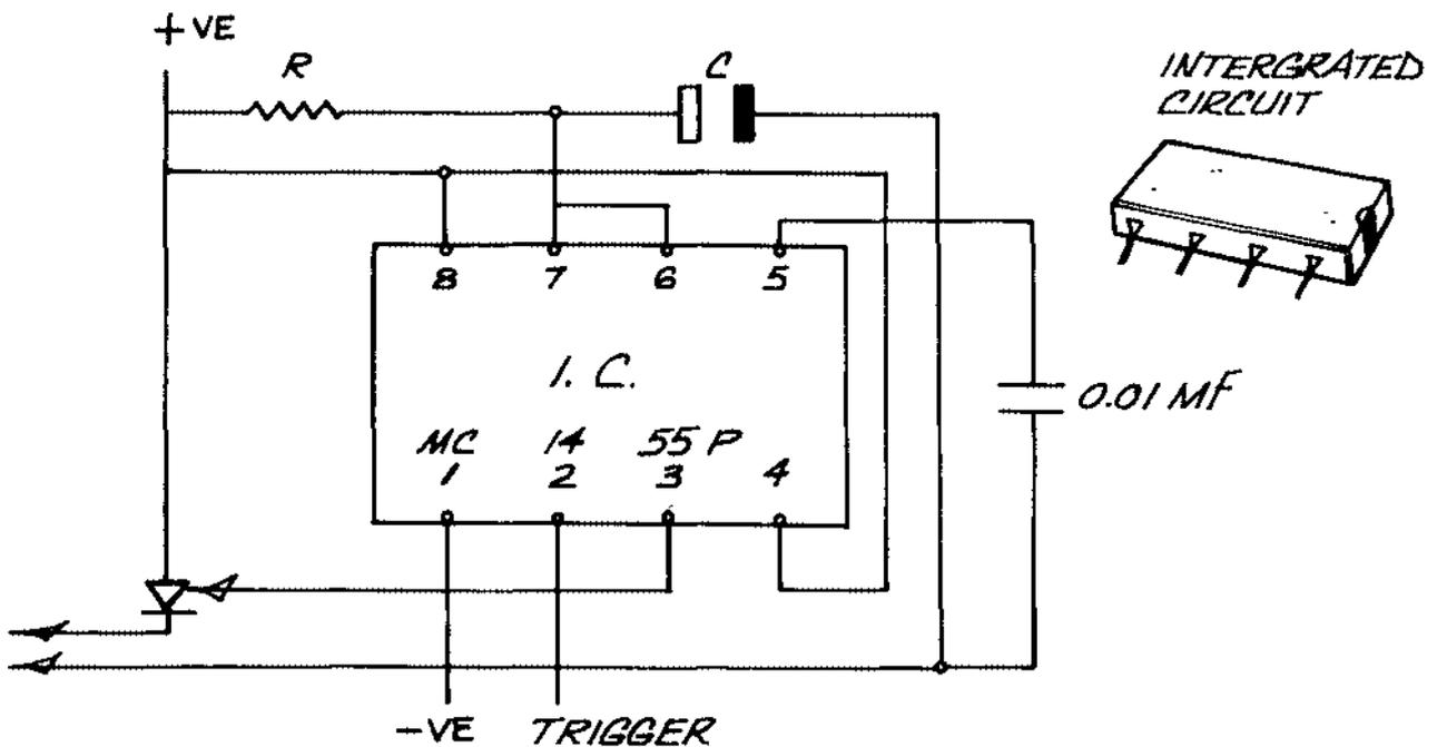
FIG. 73 INTERGRATED CIRCUIT DELAY
