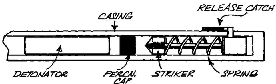
FIG. 92 SERVICE-TYPE RELEASE SWITCH
