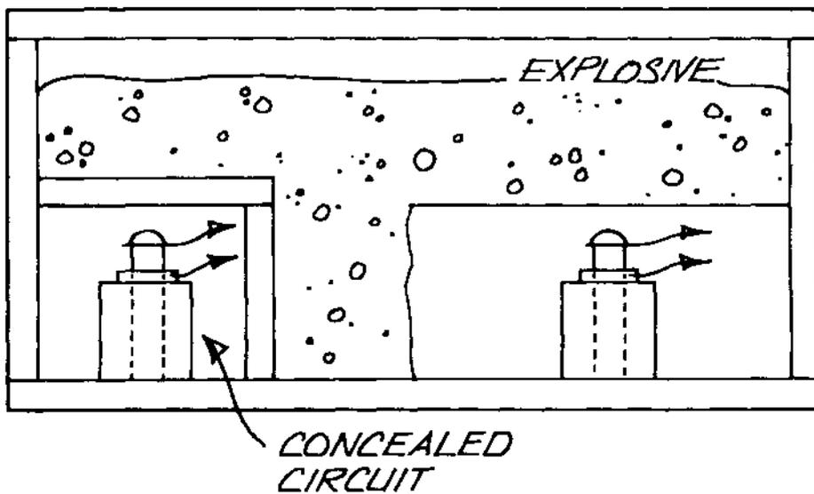
FIG. 106 DOUBLE H/LIFT SWITCH
