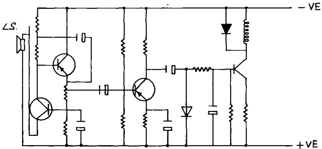
FIG. 79 ACOUSTIC SWITCH
