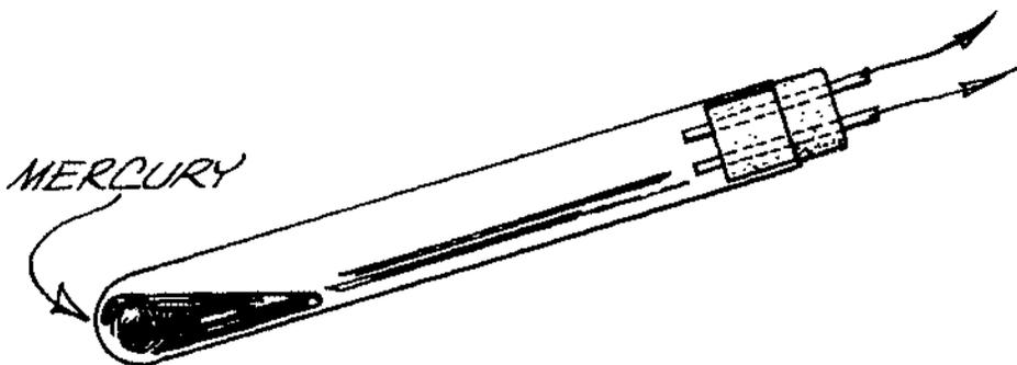
FIG. 44 HOMEMADE MERCURY SWITCH
