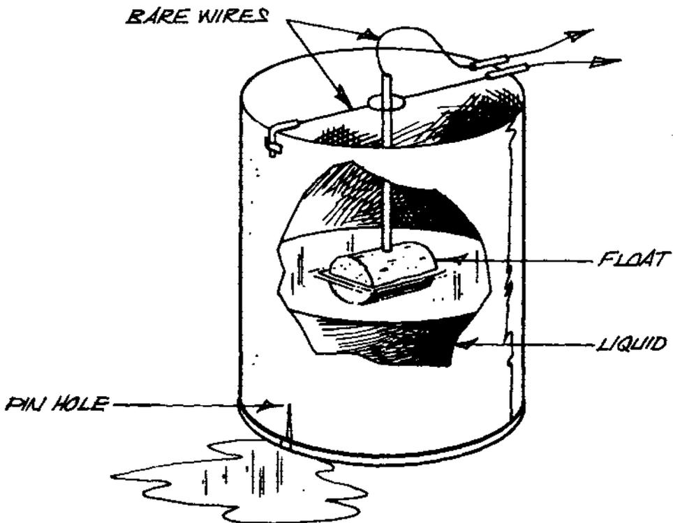
FIG. 66 WATER-DRIP DELAY
