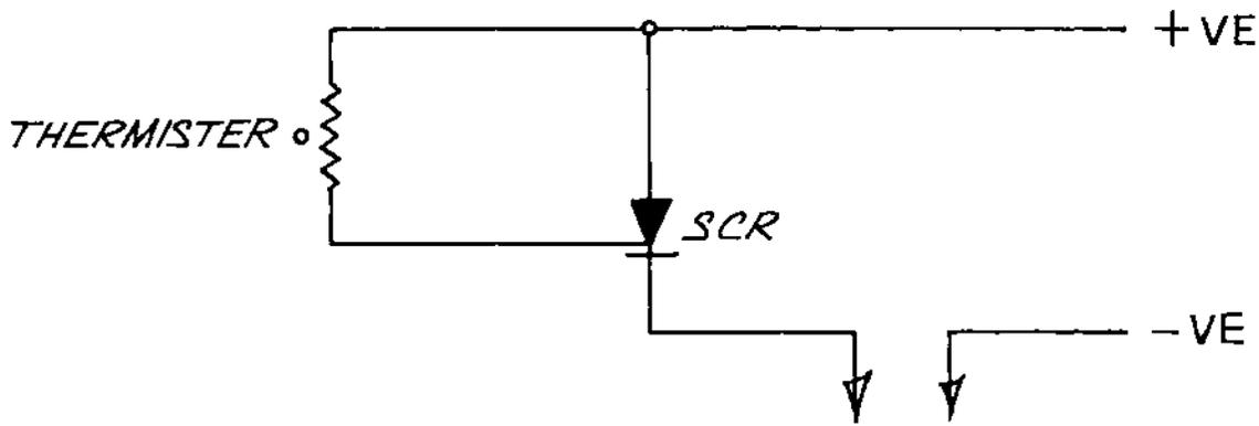
FIG. 77 TEMPERATURE-SENSITIVE SWITCH
