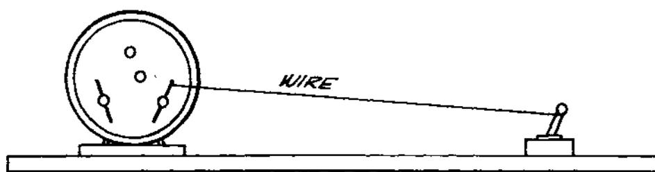
FIG. 60 ALARM WINDER & SWITCH
