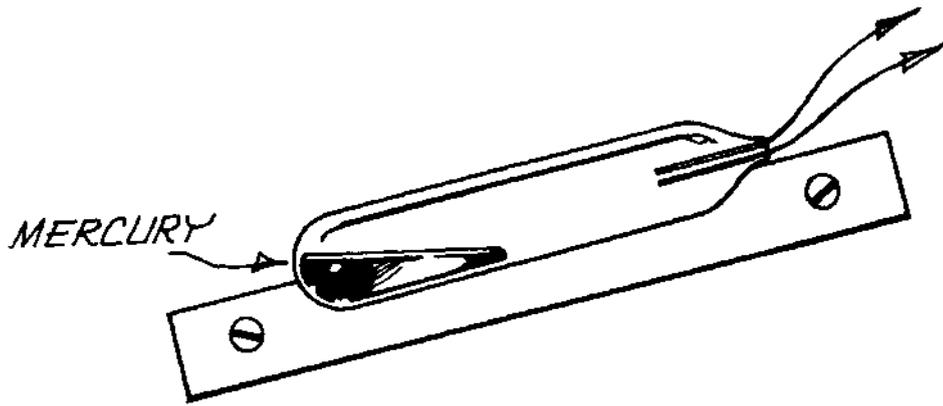
FIG. 45 COMMERCIAL MERCURY SWITCH
