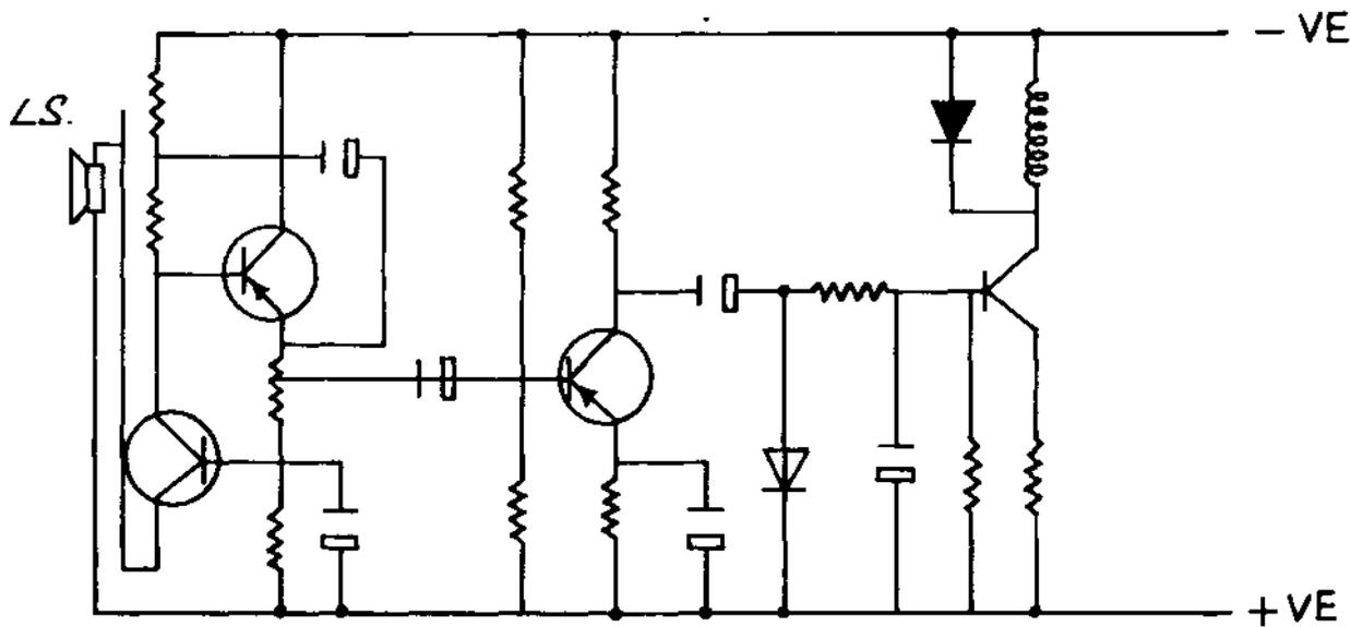
FIG. 79 ACOUSTIC SWITCH
