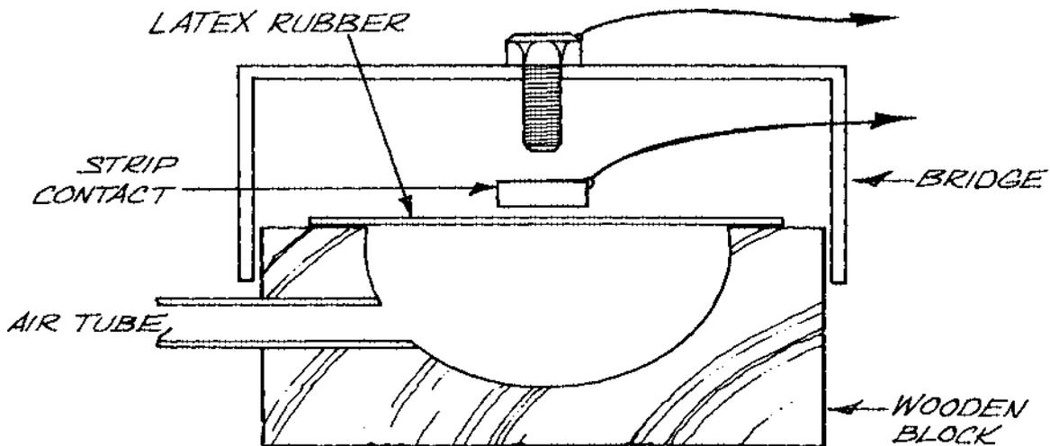
FIG. 23 PRESSURE CHAMBER SWITCH
